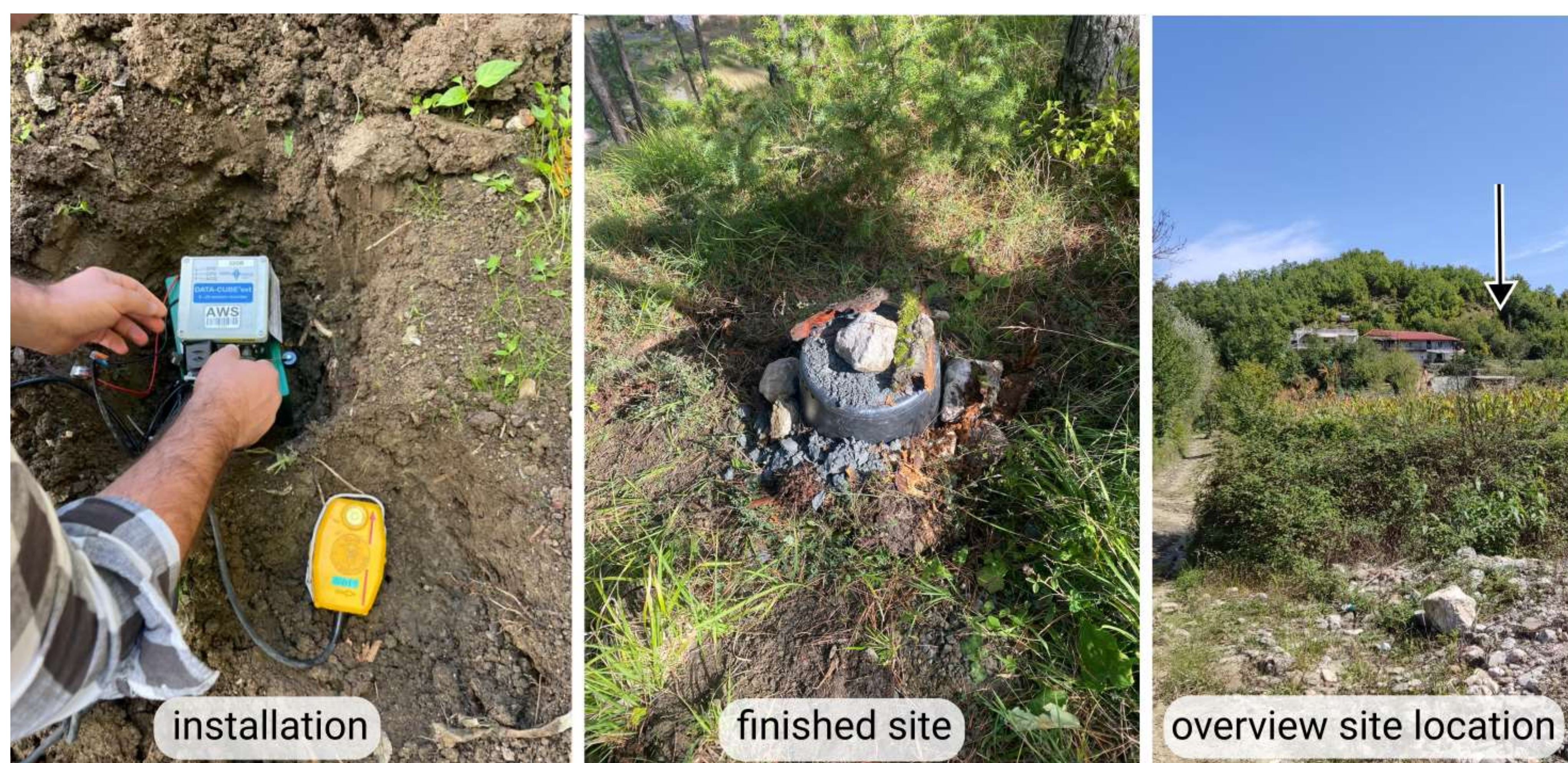
Figure 2: Example for a typical geophone installation. The geophone is buried shallowly, while the battery and the Cube data recorder are protected beneath a plastic bucket. Photo: Sofia-Katerina Kufner
