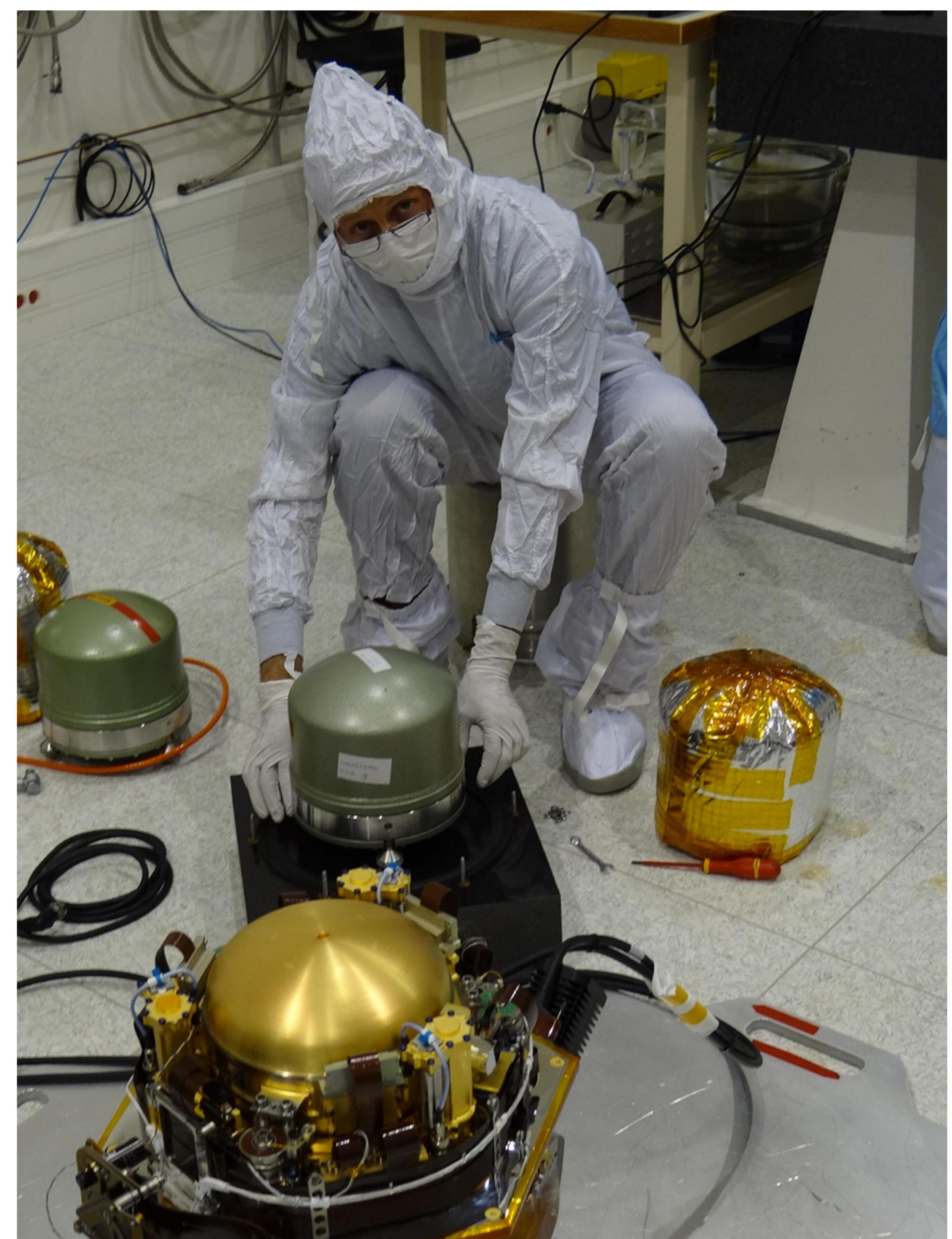
Huddle test: InSight seismometer installed next to reference STS-2.
