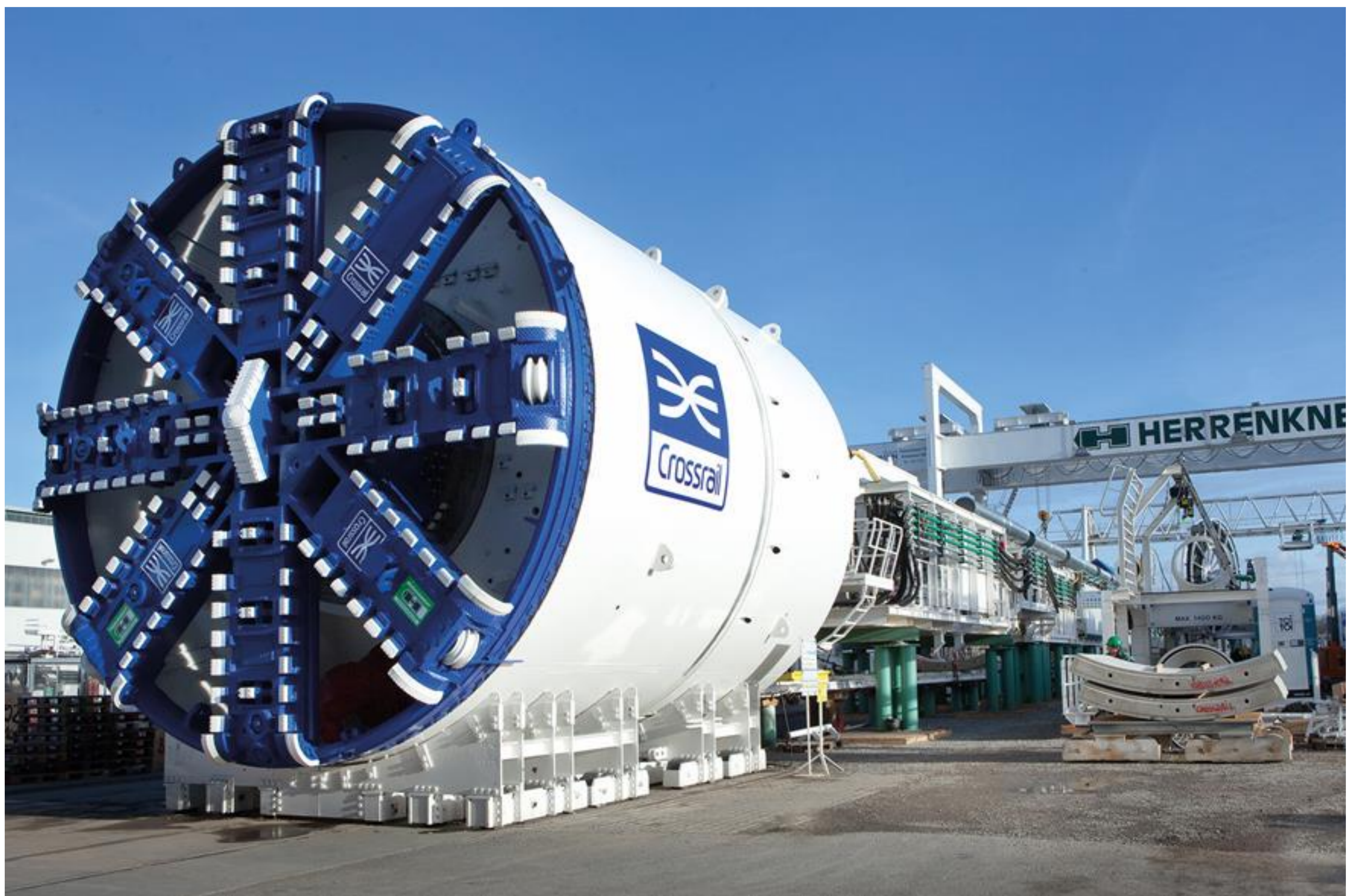
EPB shield for the Crossrail project in London with a diameter of about 7.1 meters. (source: Herrenknecht AG, www.herrenknecht.com )
