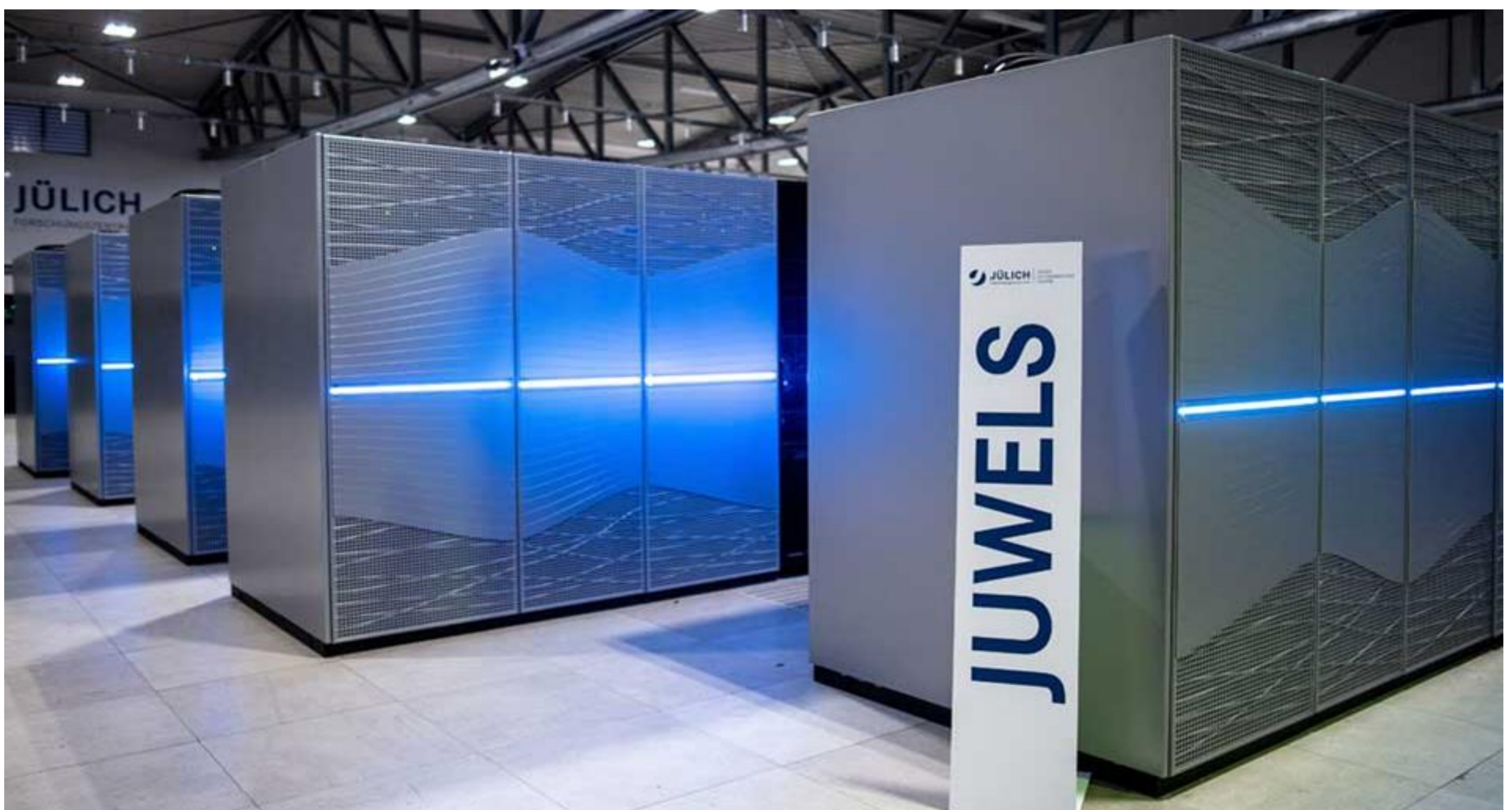
Figure 1: Performance tests of the WAVE toolbox were performed on JUWELS, a supercomputer at the Jülich Supercomputing Centre (JSC) with a total of 122,768 CPU cores and 224 GPUs.
