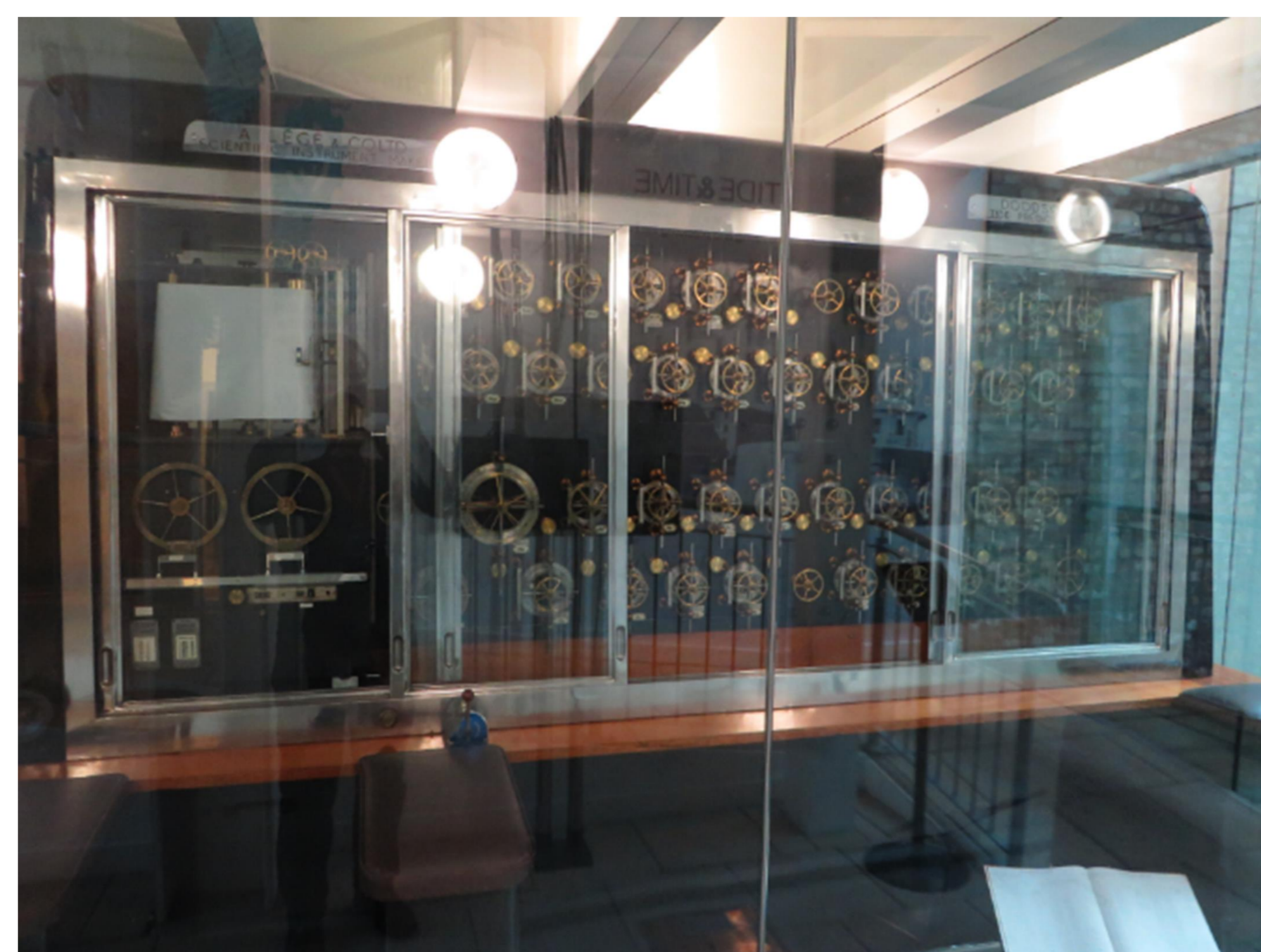
Figure 3: Doodson-Légé Tide Predicting Machine at the National Oceanography Centre, Liverpool.
